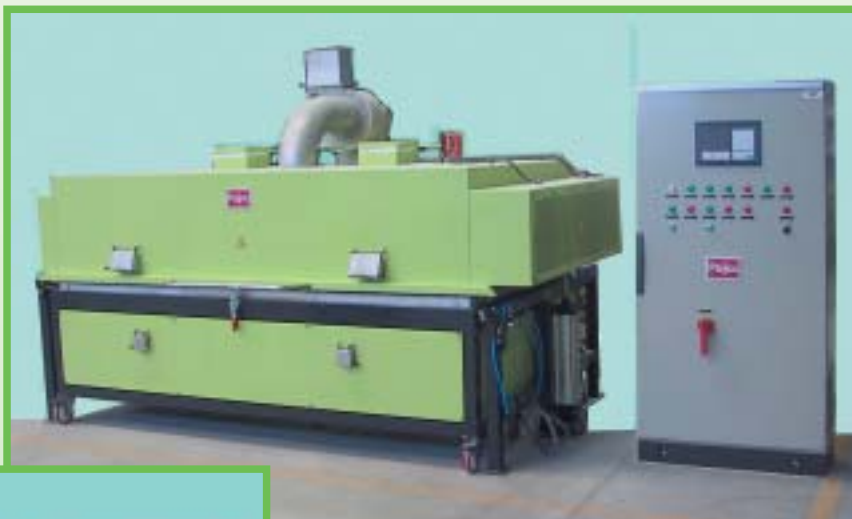
The Pujol kiln for transparent washbasins
