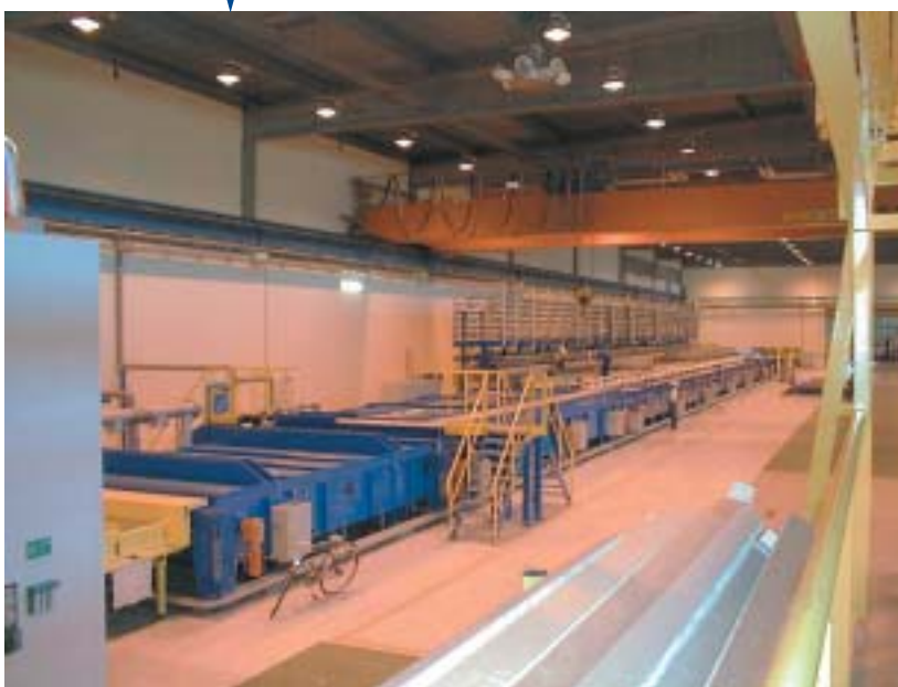
Fig. 1 - Modern architectural coater with an annual capacity of 4-5 million square metres of high performance energy saving product
