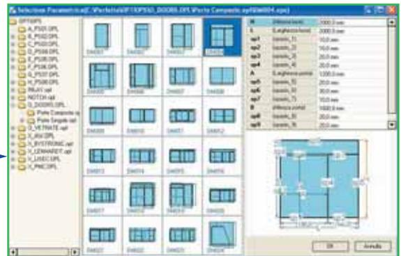
that are, in turn, also parametrical, result in a considerable number of combinations. With regards to the programme for doors, there are also libraries containing the processes needed for the assembly of the various types of frames, divided as per manufacturer.
