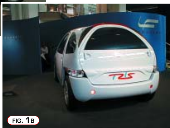
Fig. 1a-1b - Side front doors and rear window of the Fioravanti Tris have the same shape and dimension
