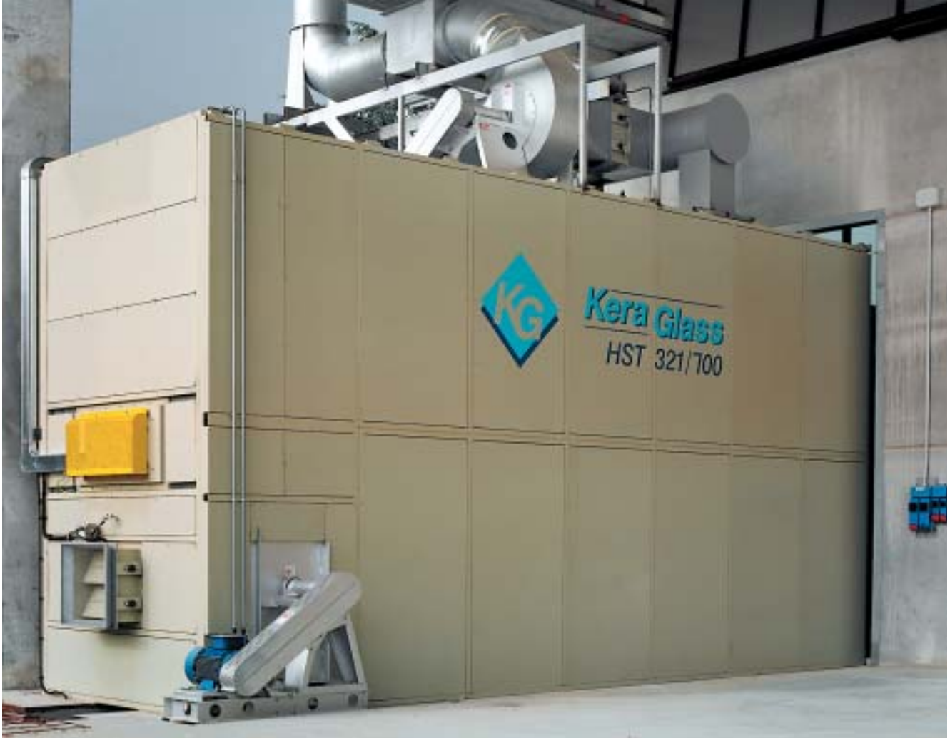
HST 321/700 Heat Soak plant
