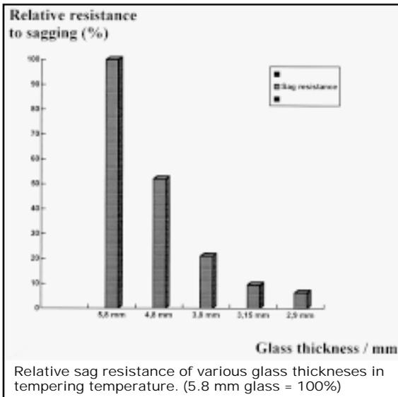
Fig. 2 Glass bending resistance as a function of glass thickness in tempering temperatures
