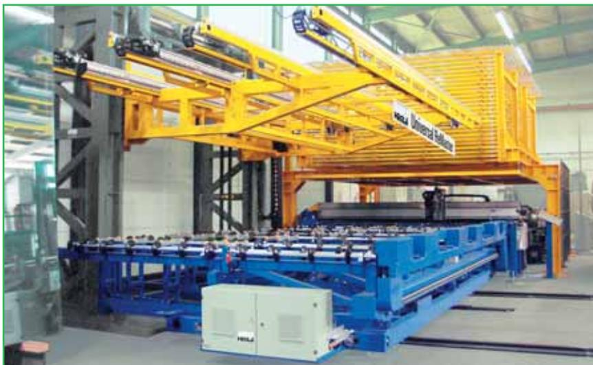
Lifting and transport frame and horizontal buffer
