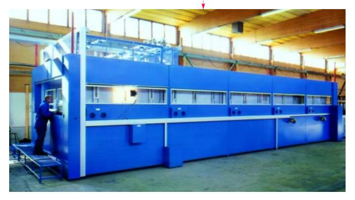
Glass-Technology International 5/2001 www.glassonline.com chamber. It is suitable for short production runs, it offers good shape control and tooling costs are low. There are, however, some disadvantages: repetition is poor; yield depends on the production mix; it is a labourintensive operation; considerable floor space is needed to house several furnaces at once.
