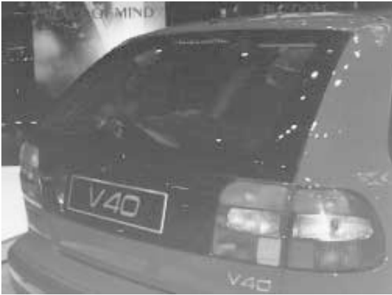
Fig. 11 Backlight peripheral border matching body design on Volvo V40
