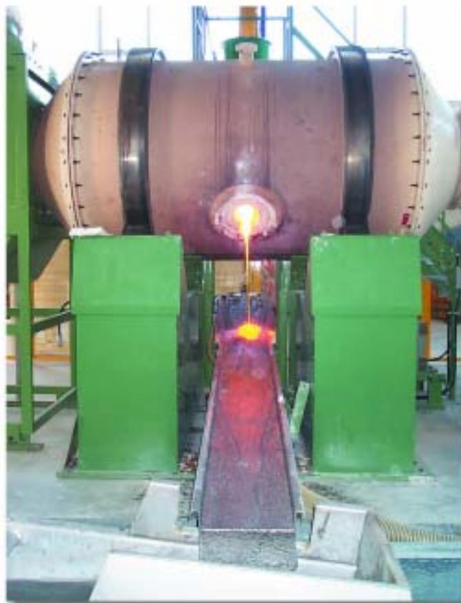
Detail of the new furnace, showing casting of liquid glass for frit production
