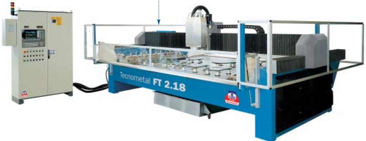
FT 2.18 Multifunctional workcentre with three or four interpolated axes
