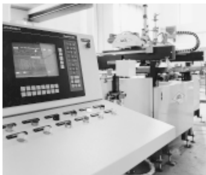
Fig. 3 The fully automatic GHS 31-S with PLC display
