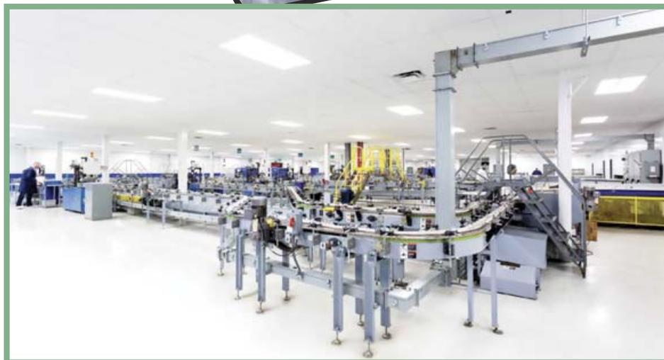
the only plant in the US manufacturing type I borosilicate glass for moulded pharmaceutical packaging products. This type of glass is suitable for very sensitive pharmaceuticals such as injectable drugs because of its excellent hydrolytic resistance and low alkaline leach rate. Gerresheimer has five other moulded glass plants in addition to the US
