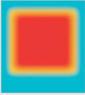
Temperature gradation with conventional metal spacer: highly distinctive thermal bridges.
