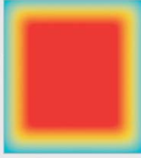
Window with thermal insulating spacer: less thermal bridges and therefore balanced temperature distribution even to the edges of the surface.
