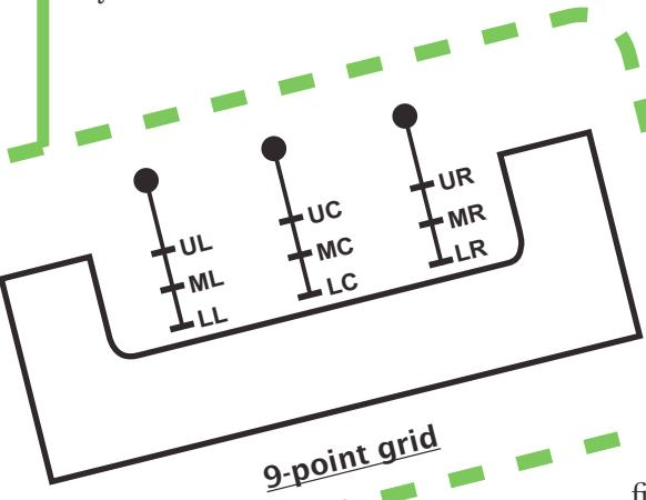
For the 9-point grid, six positive horizontal temperature differences ' $\Delta H$ ' are calculated from the values
