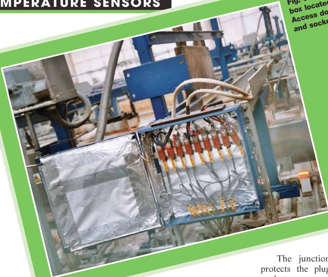
**Fig. 3 - Thermocouple junction box located at side of forehearth. Access door is open to show plug and socket connections**
