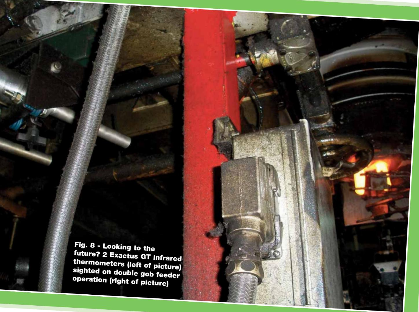
**Fig. 8 - Looking to the future? 2 Exactus GT infrared thermometers (left of picture) sighted on double gob feeder operation (right of picture)**
