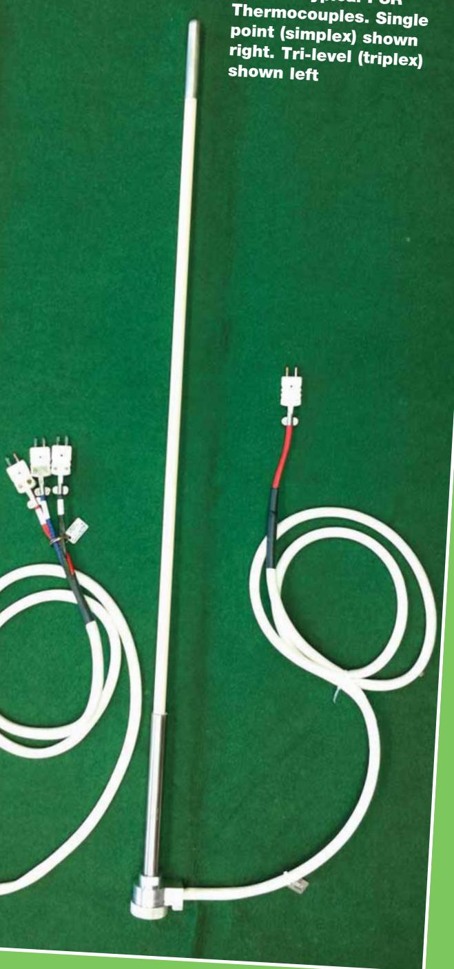
**Fig. 4 - Typical PSR Thermocouples. Single point (simplex) shown right. Tri-level (triplex) shown left**
