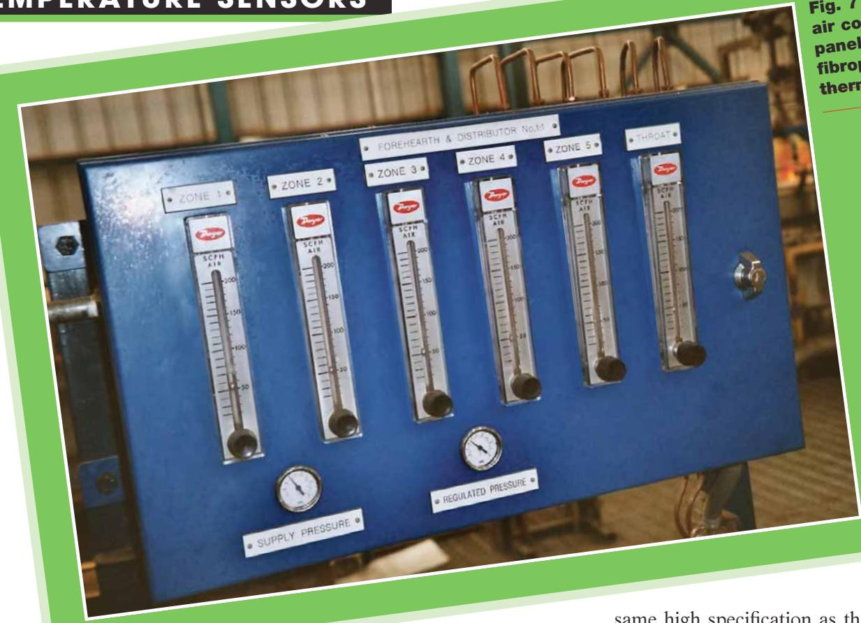
**Fig. 7 - Purge air control panel for 6 fibroptic thermometers**
