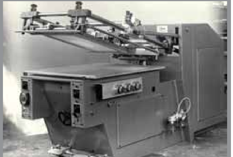
A Cugher Glass screen printing machine of the 1970s
