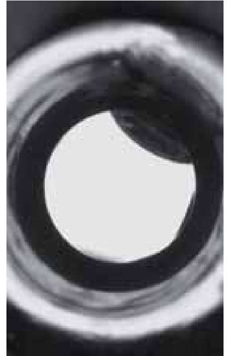
NCG distortion defect detected
